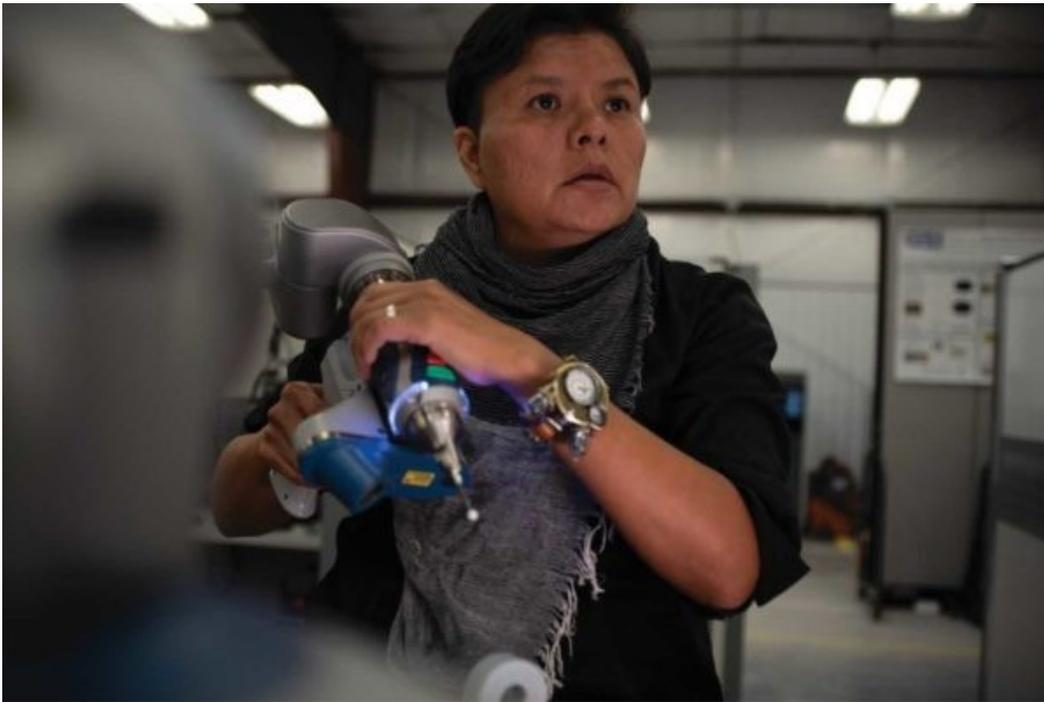
Marcie Vandever of Thoreau, NM operates the Faro Tracker Arm while conducting measurements of a 3D printed object. Metrology will be an important focus of NTU's new Center for Advanced Manufacturing.
